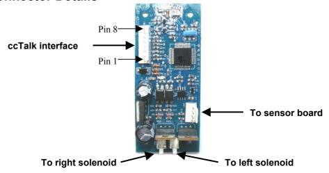
• **4.1** The coin escrow uses ccTalk interface with an 8-pin connector.
